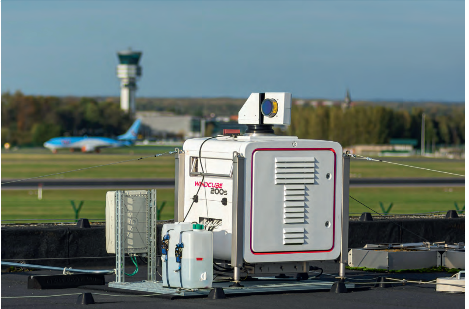
New technology: a LIDAR (laser imaging detection and ranging) radar was put into use. This radar measures the wind speed and direction at different heights.
