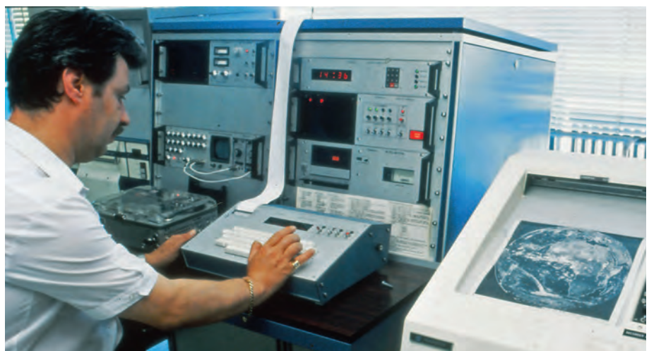
The Tecnavia Skyceiver equipment used for receiving and printing satellite weather images
