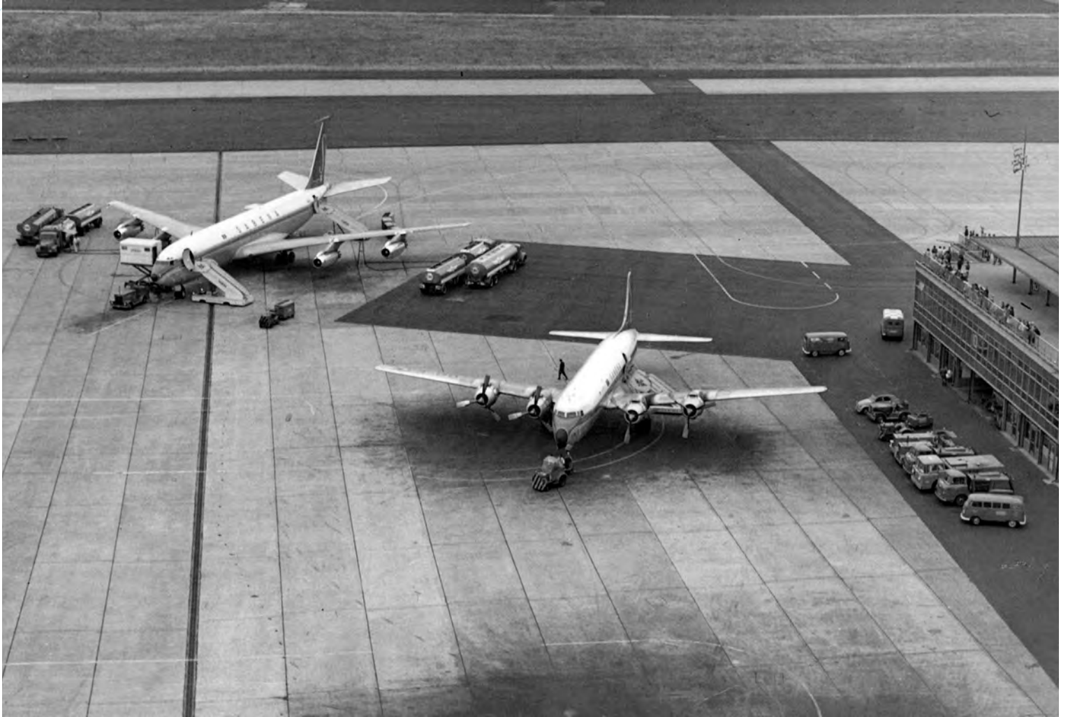
A quantum leap: from the Douglas DC-7C (right) to the Boeing 707 (left)
