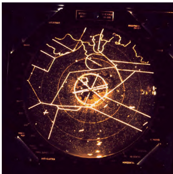
For the first time the traffic controller gets a radar map on his display.
