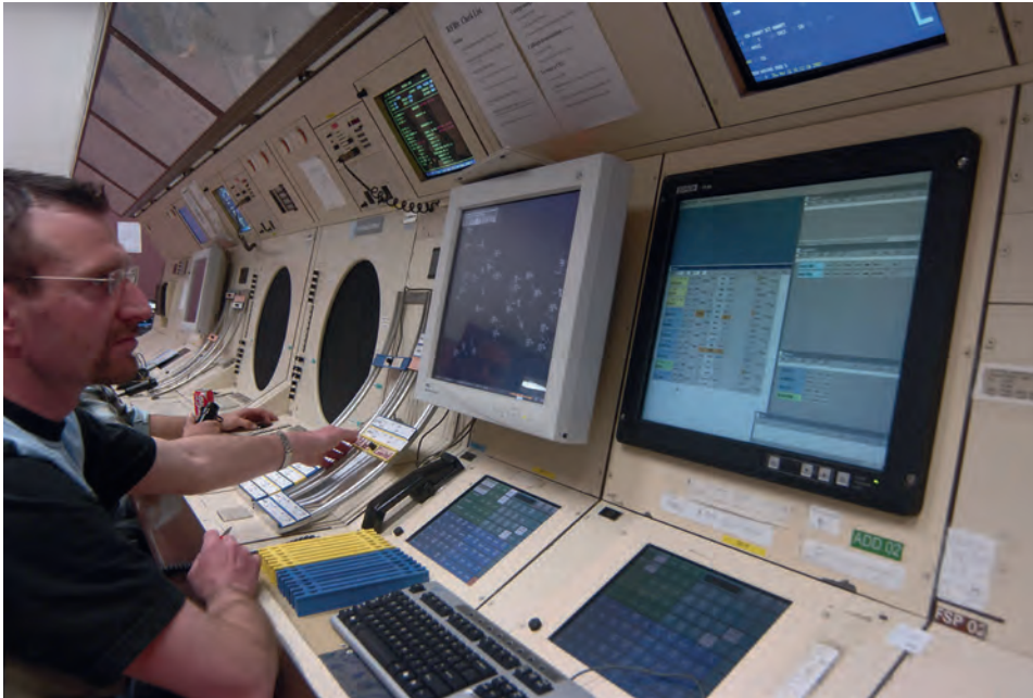
The duplicated radar screen (left) and the AMS screen (right) on the controller's workstation
