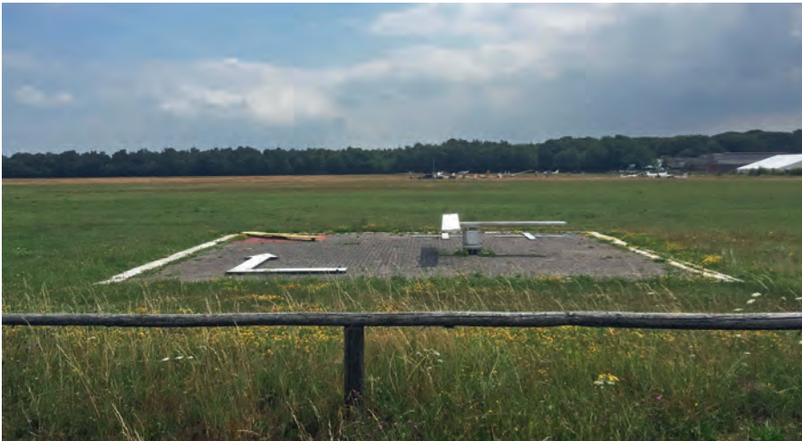
The Signal Square, or signal area, contains symbols to indicate visually to over-flying aircraft conditions on the aerodrome.
