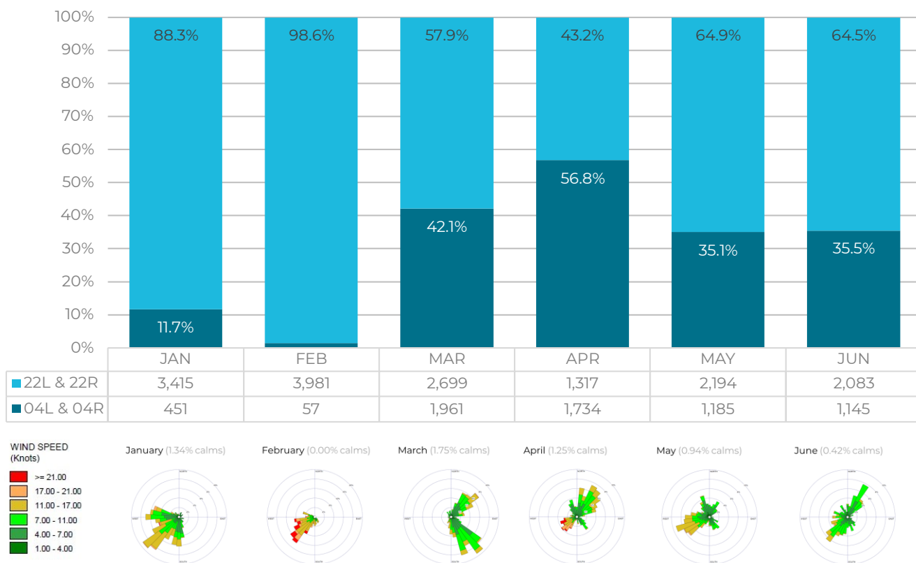
Figure 1.12: Runway use per month in 2022 (22L & 22R and 04L & 04R combined) and monthly wind roses
